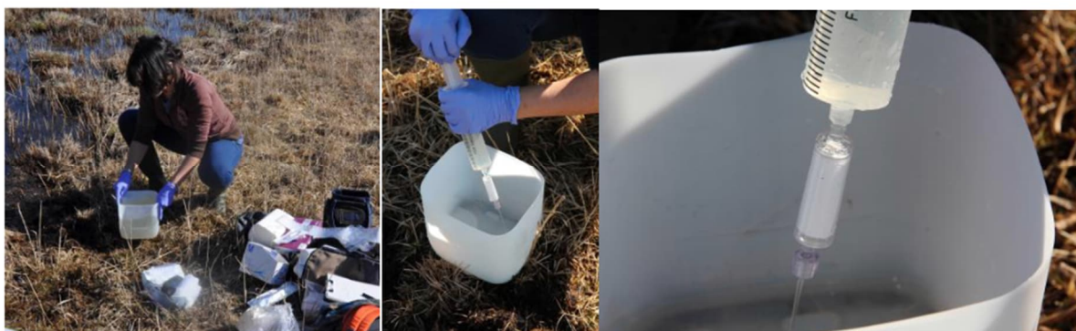
Figure 1. Phases of the sampling protocol. From left to right: collection and mixing of approximately 5 L of water (point 2), filtration (point 3), and detail of the syringe and Sterivex filter used.
